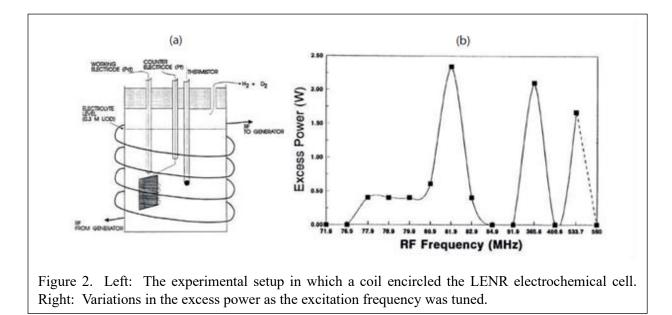
It shows on the left a schematic of the experimental electrochemical cell surrounded by a coil to introduce RF frequencies into the cell. The variations in the produced nuclear power are in the graph on the right. The RF excitation might influence either or both the electrolysis and nuclear reaction rates. The ICIQ experiments should help separate the two effects.
