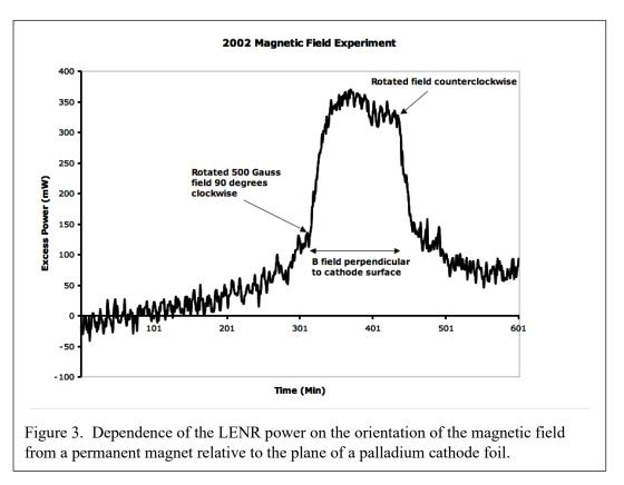
data. It is not known yet if the improvement with rotation of the magnetic field relative to the planar cathode surface was an electrolysis effect or a nuclear effect. However, the ICIQ experiments are expect to resolve that question.
